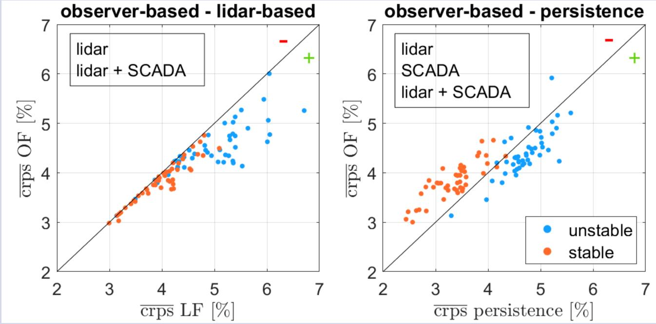
$\rightarrow$  Persistence can be outperformed for most turbines during unstable atmospheric conditions
