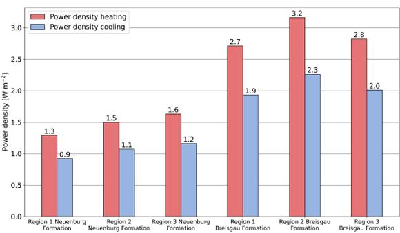
Fig. 4: ATES power densities for 2-doublet systems (Neuenburg Formation) and for 3-doublet systems (Breisgau Formation).
