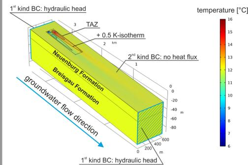
Fig. 2: Exemplary box model of a 2-doublet ATES system in the Neuenburg Formation. The TAZ around the  $\pm 0.5$  K-isotherms after 30 years of operation is highlighted.
