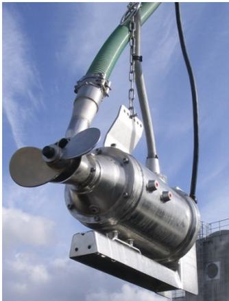
Halia Propeller System as used for 3 of 4 dissolution devices during the trial (image shows stainless steel version)
