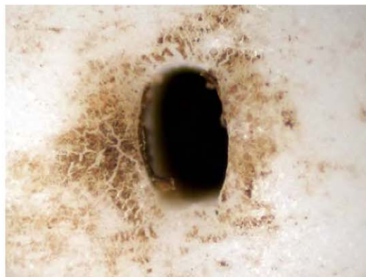
Figure 10: Silicone-membrane after one year operation in a wastewater treatment plant
