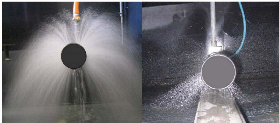
Figure 2 – Outgassing behavior of a new (left) and a coated diffuser (right)
