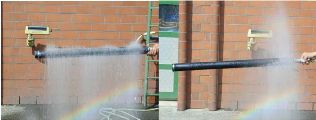
Figure 2: Outgasing of a new and a biologically coated EPDM-membrane diffuser
